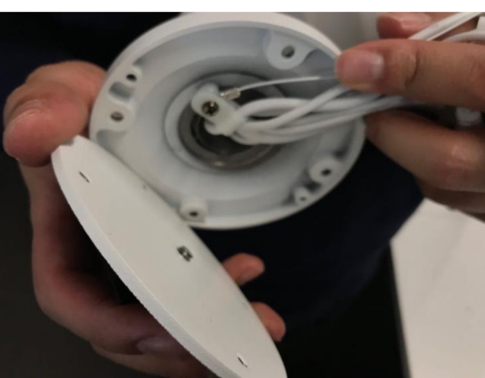
B. Fix the adapter on the camera
