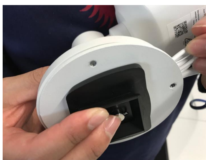
B. Fix the adapter on the camera
