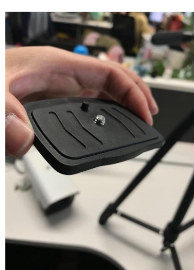
A. Tripod connector fixed on the adapter
