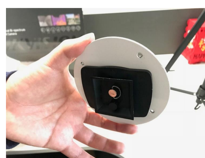
A. Tripod connector fixed on the adapter
