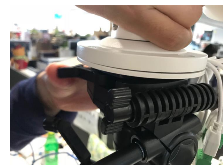
C. Install the camera on the tripod
